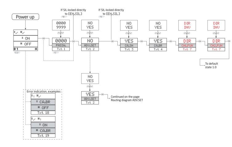
\*1.0 Default state. Line 1 shows status for channel 1 and channel 2. Line 2 shows status for sensor 1. Line 3 shows status for sensor 2.
